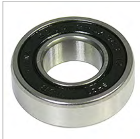
10032786 BEARING,SEALED,ENT DOOR,6203-2RSQ-3/4,ZWZ
