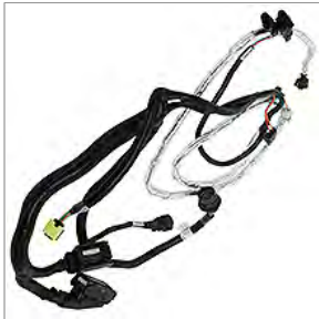
10010494 HARNESS,WRG,DCU CONTROLS,ISB10 BBCV
