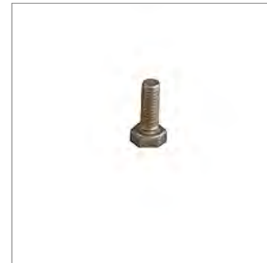
5010279A (Webasto® 5010279A) BOLT HEX HD M6-1.0(6G)X16 (8.8) ZP (DIN 933) OLD# 267279 & 9012677A
