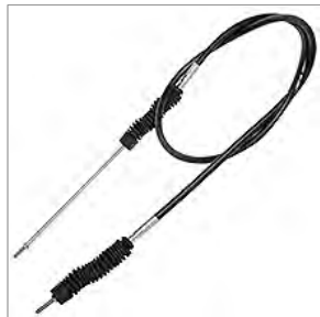
01857192 CABLE,30C ACCEL,66 LG,MORSE 310612 CS/TCFE
