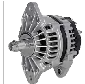
8600313 (DelcoRemy® 8600313) ALTERNATOR 28SI 12V 200A
