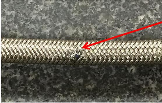
Steel braid has been damaged, fuel line **MUST** be replaced.
