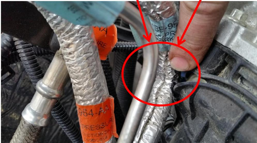
4. Inspect for clearance between the fuel lines and the air intake tube.
