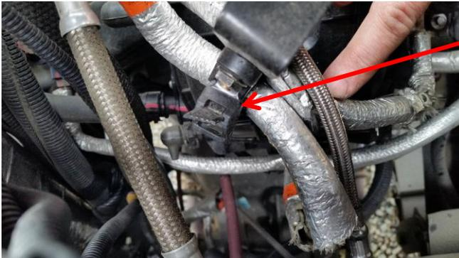
Cable tie and heavy duty cable mounts
