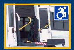
Special needs Micro Bird with double-leaf wheelchair doors offer protection on both sides of the lift, thus adding to passenger safety, while offering superior weather seal and door strength.
