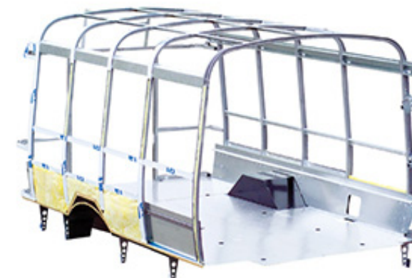
Insulated steel roof bows provide the backbone of the passenger safety cage
