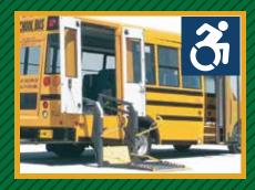
Special needs Micro Bird with double-leaf wheelchair doors offer protection on both sides of the lift, thus adding to passenger safety, while offering superior weather seal and door strength.
